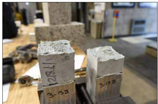
Figure 4: Newer products, such as Ultra-High-Performance Concrete (UHPC) can offer new benefits, but pose risks as codes, specifications, and testing procedures that are appropriate for traditional concrete may not work for UHPC.
